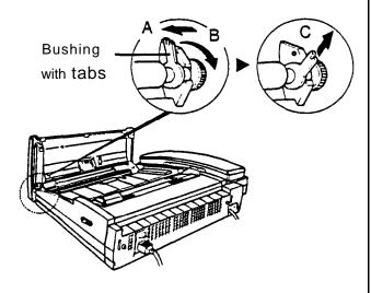
**lote:** Be careful not to lose the bushing on one and of the roller when disassembling.
